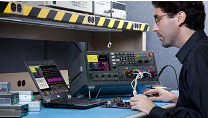
Figure 2 The Keysight N6705C DC Power Analyzer, outfitted with a Keysight N6781A Battery Drain Analyzer module and BV9201B PathWave BenchVue Advanced Power Control and Analysis Software, provides a complete instrumentation solution for performing battery rundown tests.
