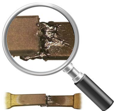
Bad contact weld due to switching very high current
