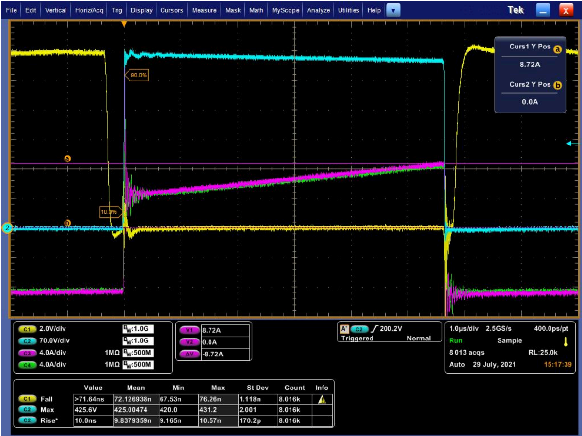
Fig. 12. System running in BUCK mode - GaN FET high-side currents
