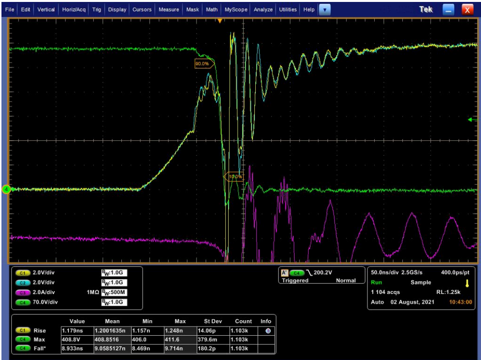
Fig. 16. Zoom of Q2 and Q4 low-side GaN FETs - switch ON
