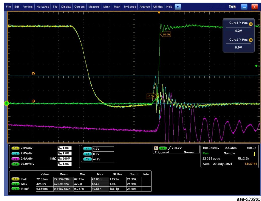
Fig. 11. Zoom of Q2 and Q4 low-side GaN FETs - switch OFF
