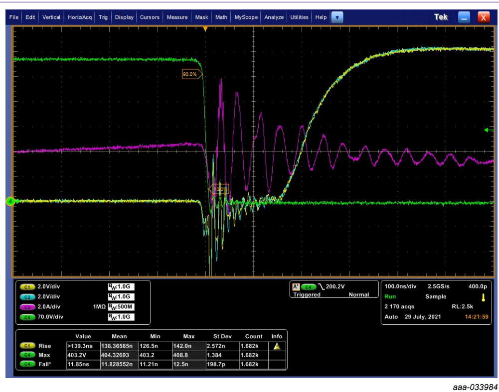
Fig. 10. Zoom of Q2 and Q4 low-side GaN FETs - switch ON
