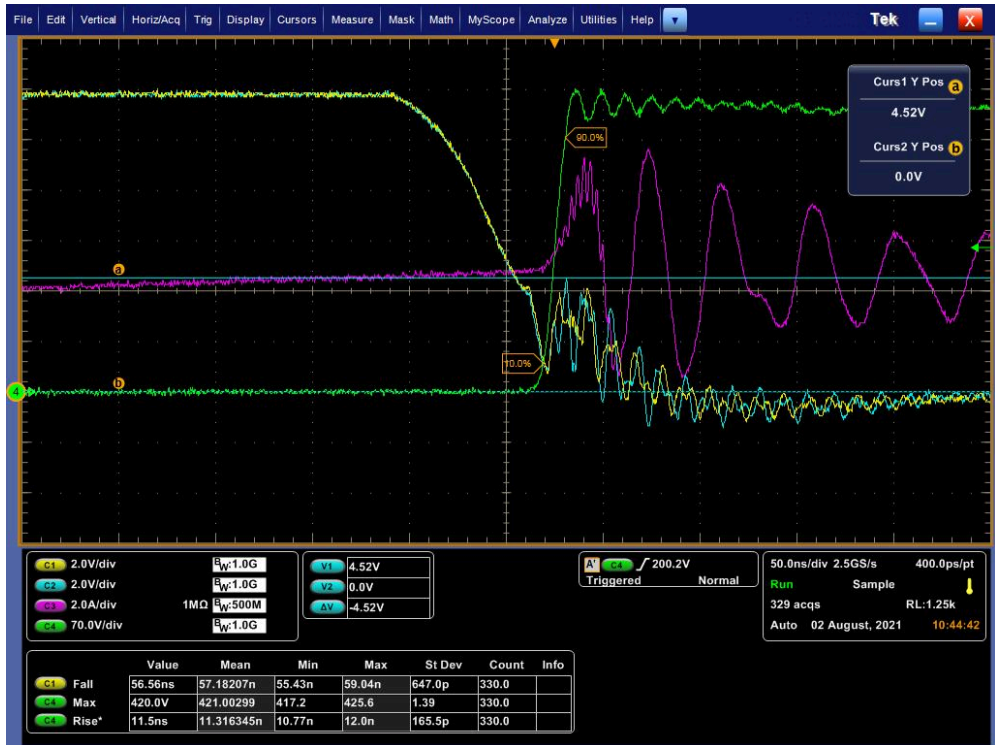
Fig. 16. Zoom of Q2 and Q4 low-side GaN FETs - switch ON
