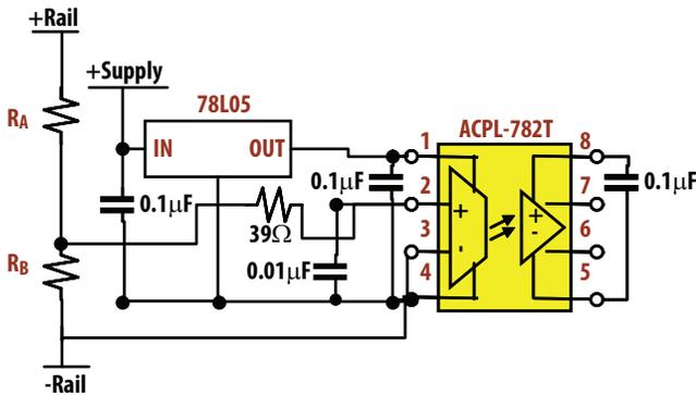
Figure 2. Stepping down the High Rail Voltage to match the Input Voltage Range of ACPL-782T
