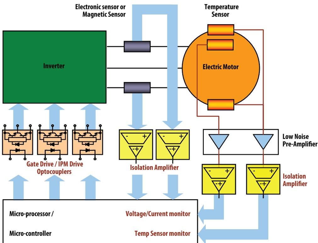
Figure 1. HEV Electric Motor Drive System
