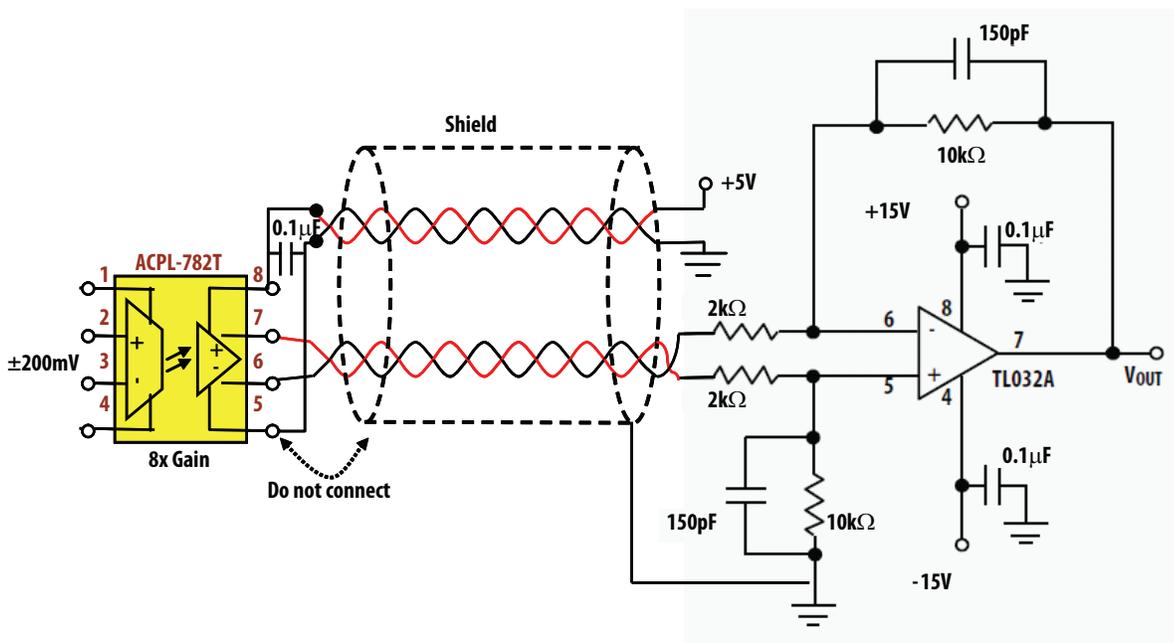
Figure 4. Remote Voltage Sensing Configuration with ACPL-782T
