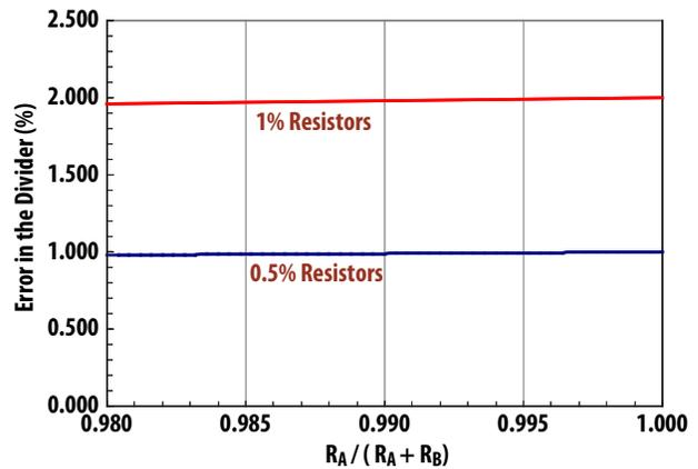
Figure 3. Divider Error for 0.5% and 1% Resistors Used
